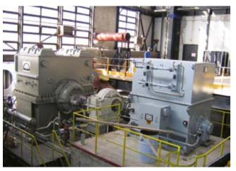
Supply: 12,000 kW, 6000 V, 4 poles, frame 800 Application: Centrifugal compressor
