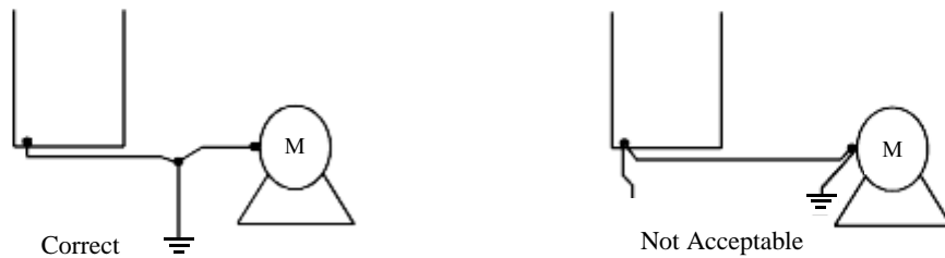
Grounding of IMPULULSE VG+ Series 3 Drive and Vector Control Motor
